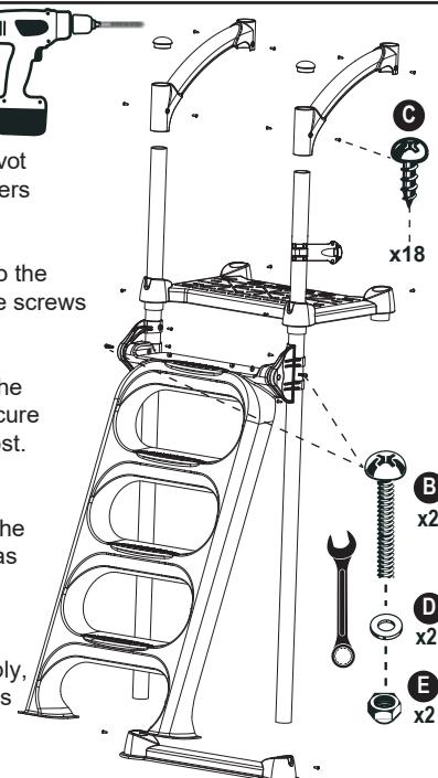
Use sliding lock as a guide to drill hole into ladder in up position. Use a 3/8" drill bit with a cordless drill.
