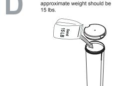
2) Screw the lid in place and align the cover ribs with the holes in the ballast base.
